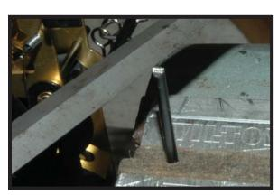
One should than be sure to file down the cut end of the wire for the sharp edges can take a nice slide in one of your fingers.
