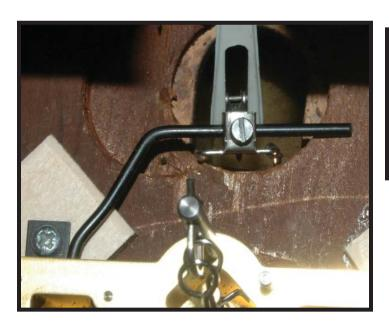
Here you see the perch at the proper height and the bird is properly located in the door. I usually keep them to the left a bit to prevent the bird's beak from hitting the door.
