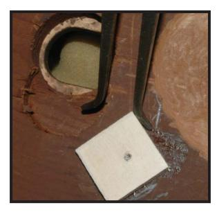
I put that line there so I could measure the distance from the top of the front plate of the movement to the location I want the perch wire to be relative to the door. I used an outside calipers as you see in the photo. I have the left caliper leg a little above the bottom of the door so the bird's feet will clear the door threshold.
