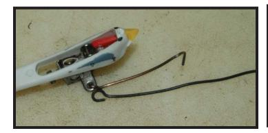
When I connected the wire from the bird to the door it worked OK but the door came only half open. I needed a new wire. This shows the old and new wires. The new one worked. The door was fully open.
