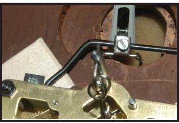
I moved the perch up a bit by bending the wire as you see here. I could not bend it at the lower 45 degree bend because that bend was too near to the top of the movement and I couldn't reach it. Thus I made do and bent it as you see here.
